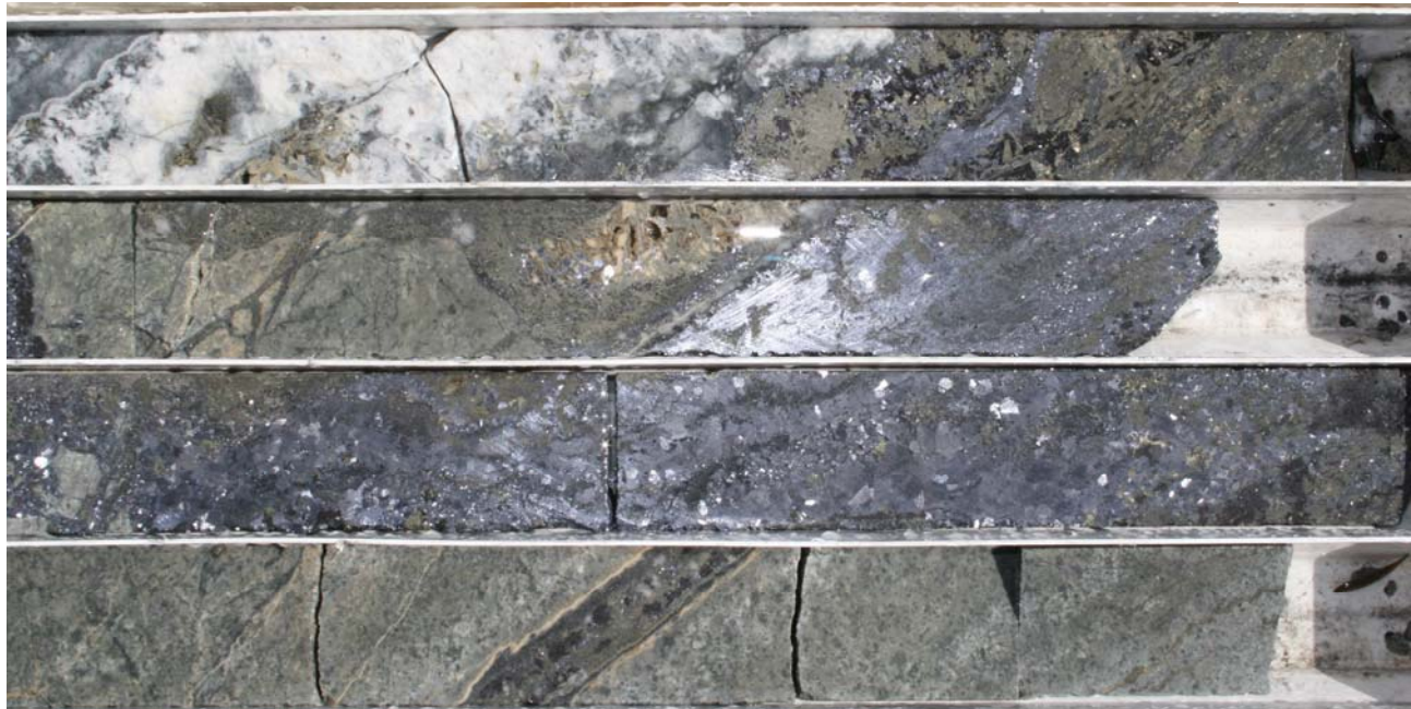
Plate 1 Digger Lode core showing high-grade argenterous (silver-rich) galena with sphalerite and quartz veins, typical of recent drill cores from the main Digger Lode, assays for which are reported on the next page.
